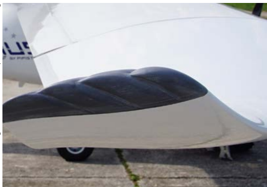
Flight tests with SEW tips on a fixed wing
