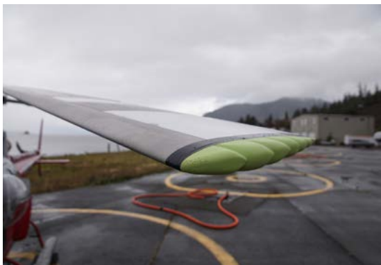
Flight tests with SEW tips on AS 350 M/R blades
