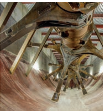
Paddle mixer unit in Dry Fermentation System
